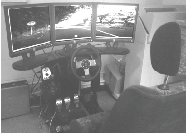
Fig. 2: Driving simulator consisting of triple-screen display, PC-based steering wheel and pedals, and car seat
