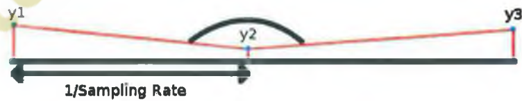
Figure 6.12: As the sampling rate decreases the angle at y_2 approaches a limit of 180 degrees.
