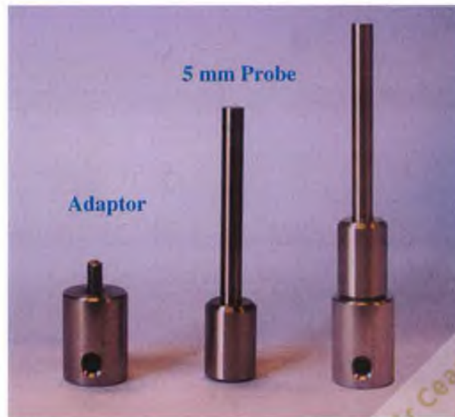
Figure 2.1: Adaptor constructed for use in the rupture testing of alginate gels. The adaptor facilitates the attachment of a 5 mm probe to the load cell of the Zwick/Roell Universal Testing Machine.
