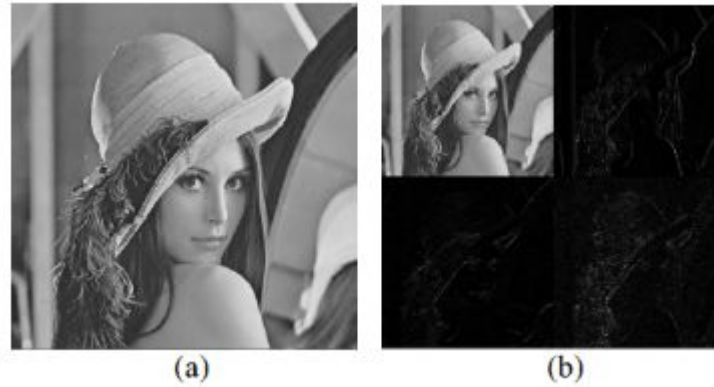
Figure 20: (a) Original image (b) After 2-D Haar DWT is applied (Chen, & Lin, 2006).
