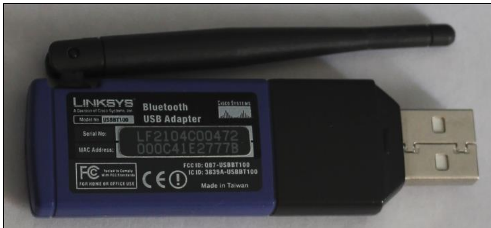
Figure 8: Linksys USBTT100 unmodified device (BD_ADDR: 00:0C:41:E2:77:7B)
