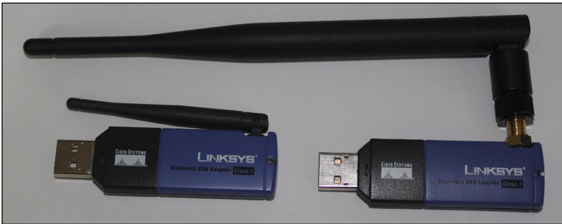
Figure 10: Linksys USBBT100 unmodified and modified devices (pigtail soldered in place)
