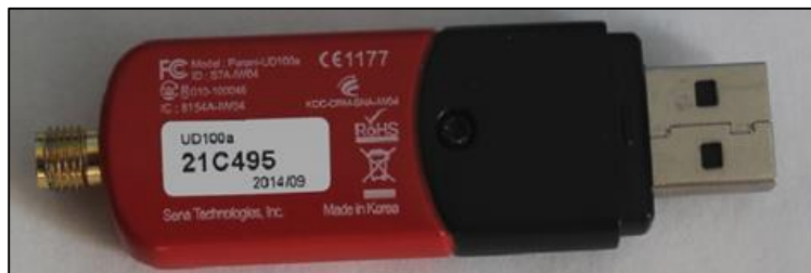
Figure 12: SEN A Device, showing Lower Address Part (LAP) - 21C495 (BD_ADDR: 00:01:95:21:C4:95)
