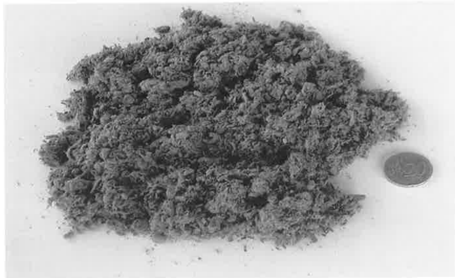
Plate 3.1 Thermally dried primary sludge from Ringsend Treatment Plant, Dublin
