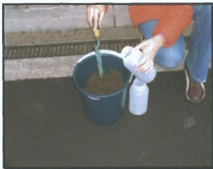
Figure 5.7 Composite sludge sample from Monaghan wastewater treatment plant
