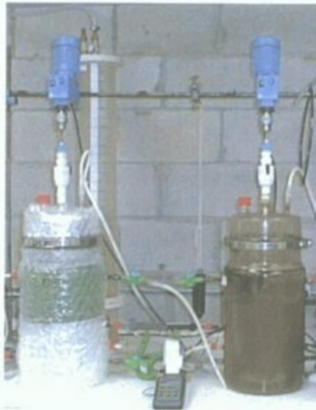
Plate 4.1 Pilot Scale Digesters in Operation
