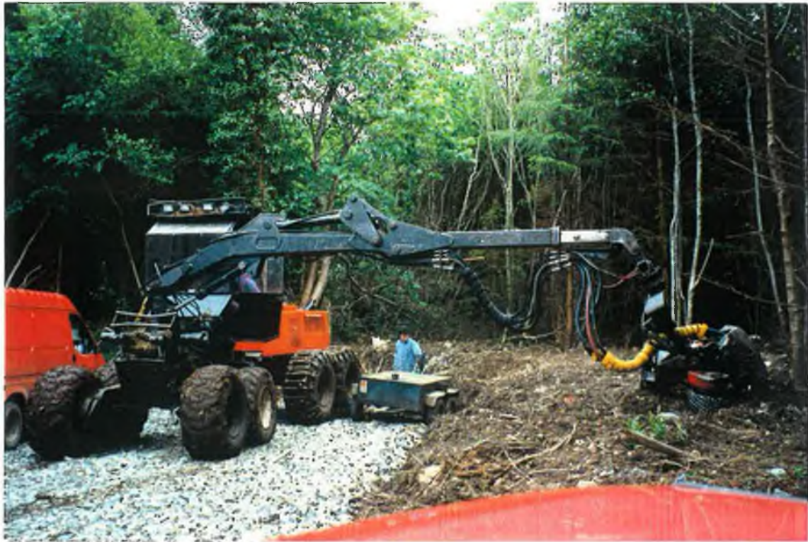
Plate No. 1:(above) The Teva Harvester with Silvatec harvesting head. A combination of band tracks and tyres were used for the harvester trials.
