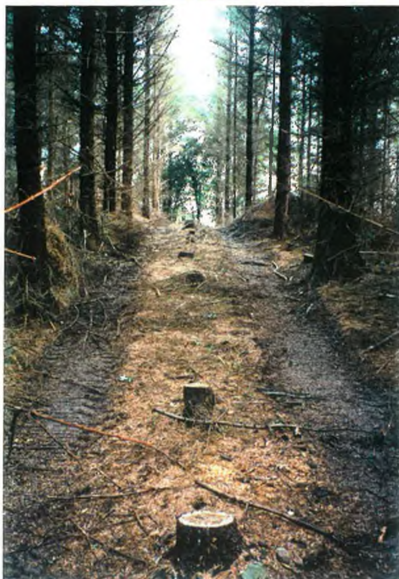
Plate No.11:(above) Plot C after the Ponsse S10 forwarder, tyres and brash. No evidence of the loaded passes can be seen.
