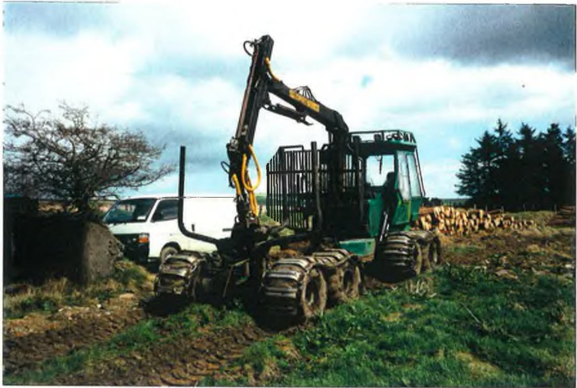
Plate No. 7:(above) The Norcar 490 forwarder. This forwarder complete with band tracks was used in the Hollyford trials.
