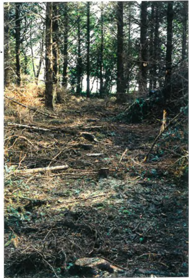
Plate No. 10:(right) Plot B after the Ponsse S10 forwarder, Band tracks & brash. No visible signs of where the wheels passed.
