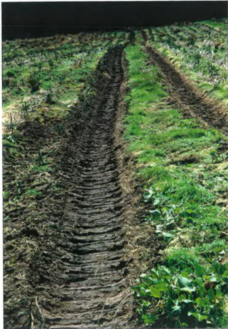
Plate No. 13: The extraction route from the forest stand to the yarding area at the roadside. Despite the dry soil conditions rutting is evident on the route after 8 loaded passes with the Norcar 490. Band tracks were essential to achieve traction and maintain mobility especially after rainfall. The rut depth is approximately 5cm deep along the length of the track and soil berms are evident on the sides of the tracks as the soil is displaced.
