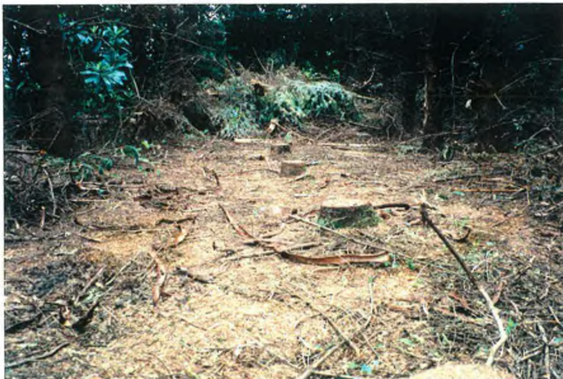
Plate No.11:(above) Plot C after the Ponsse S10 forwarder, tyres and brash. No evidence of the loaded passes can be seen.
