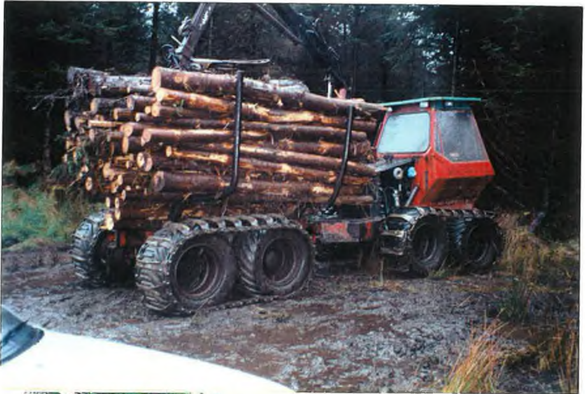
Plate No. 5:(above) The Norcar 480 forwarder used in Lissadell forest with 500mm wide band tracks.
