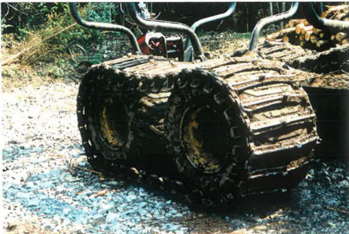
Plate No. 4:(below) The band tracks used on the Ponsse S10 Forwarder. These steel tracks are used on soft ground to improve traction, mobility and prevent the machine sinking.
