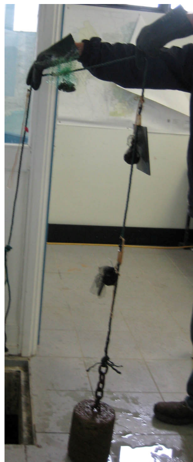
Figure 3. Bags with adult mussels and PVC juvenile settlement plates attached to the suspension rope, deployed in the drinking water treatment plant chambers (photograph by Sara Meehan).
