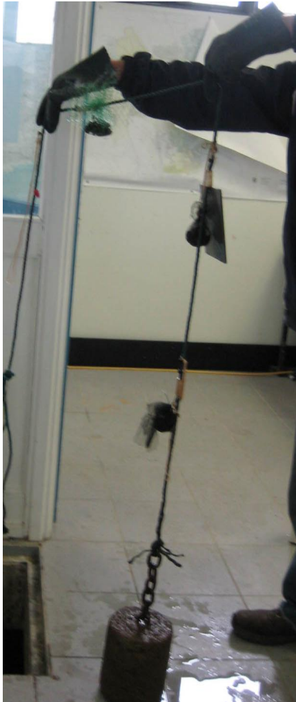
Figure 3.3 Bags with adult mussels and PVC juvenile settlement plates attached to the suspension rope, deployed in the drinking water treatment plant chambers (photo by Sara Meehan).
