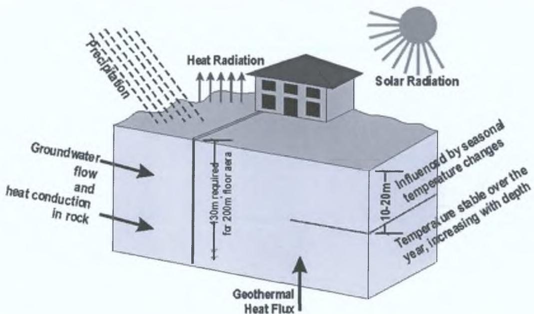
Fig. 3-2 Delivery and storage of heat energy in the ground [Sanner, 2002]
