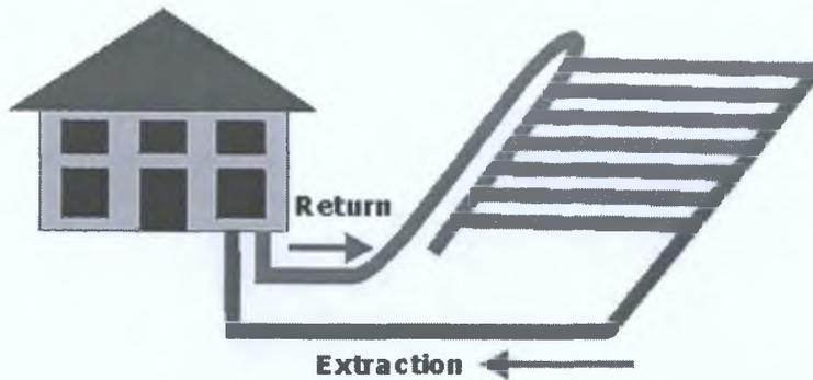
**Fig. 3-6 Horizontal closed loop collector in parallel**
