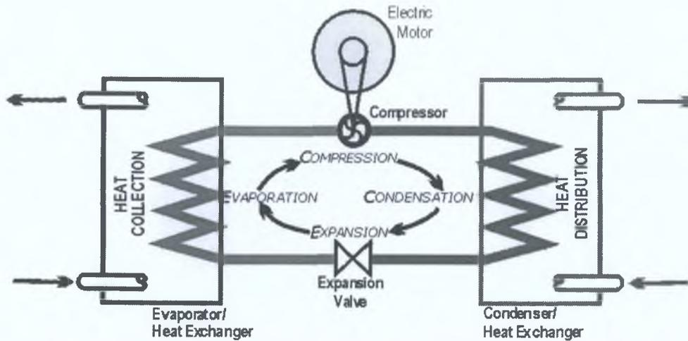
**Fig. 3-3 How a heat pump works**
