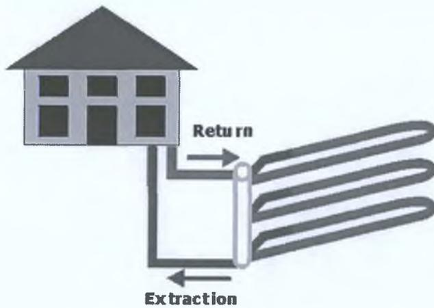
**Fig. 3-7 Horizontal closed loop trench collector**
