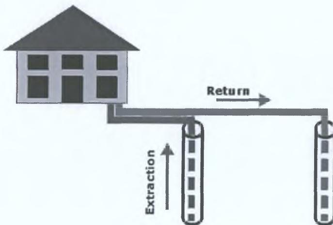
**Fig. 3-4 Open loop (Doublette) system**
