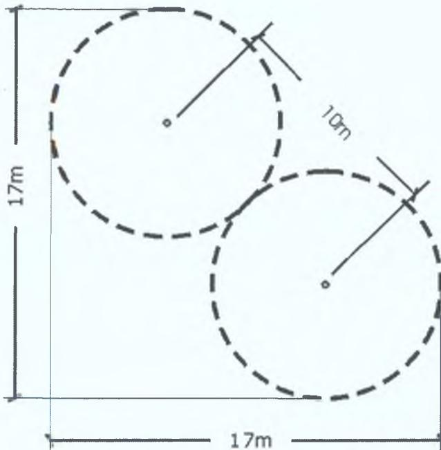
**Fig. 5-2 Borehole spacing for individual collectors**
