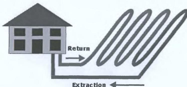
**Fig. 3-5 Horizontal closed loop collector in series**
