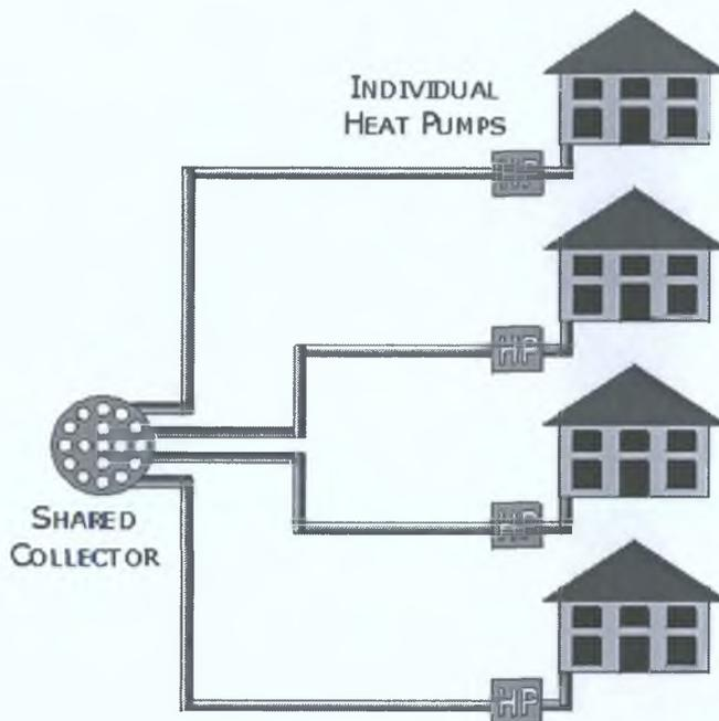
**Fig. 4-2 A shared collector system distributing low grade heat to individual heat pumps at each house**
