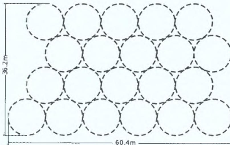
**Fig. 5-1 Borehole spacing for a shared collector**
