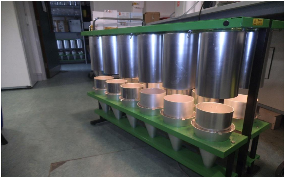
Plate 3.6: Bank of Berlese-Tullgren Funnel used for extraction of micro-invertebrates
