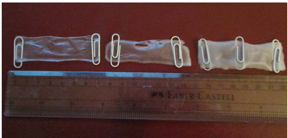
Figure 15 Left to Right; a visual representation of polycaprolactone films manufactured through solvent cast method from 4%, 8% and 10% w/v concentrated solutions
