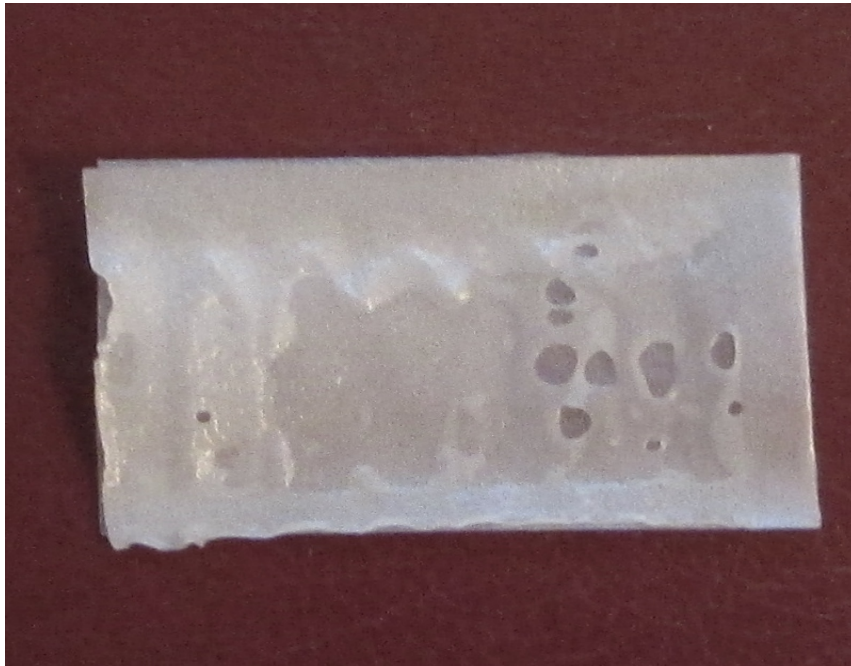
Figure 32 Defects on sample due to Insufficient cooling time
