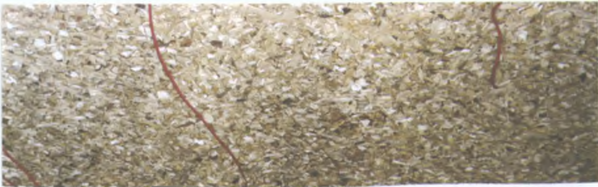
Plate 2.12: Wood Chipping Used As Bedding Material At Toomevara STP, Co Tipperary.
