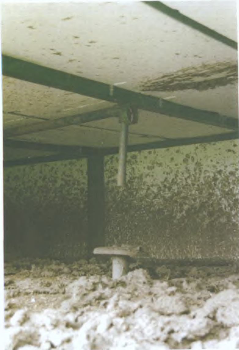
Plate 2.11: Liquid Sludge Distributed By Splash Plate
