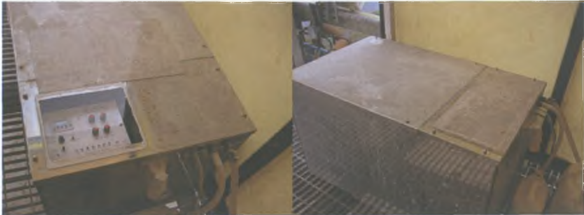
Plate 3.3 The Bio-reactor installed to determine effectiveness of bacterial addition to remove hydrogen sulphide
