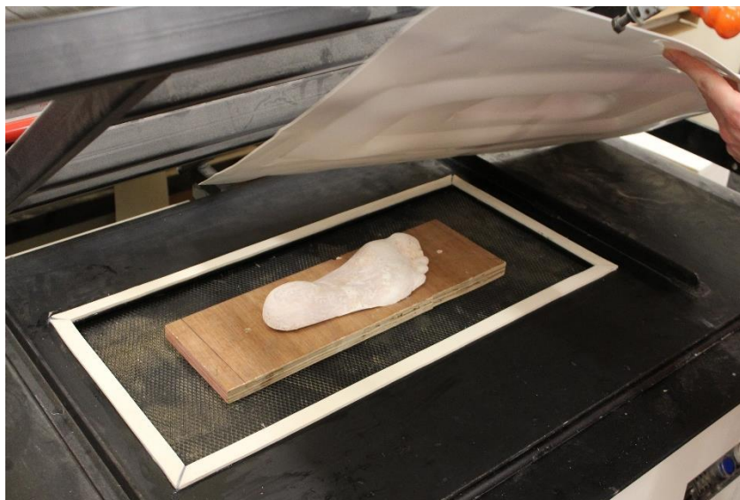
Figure 42: Vacuum moulding of the plaster cast model.
