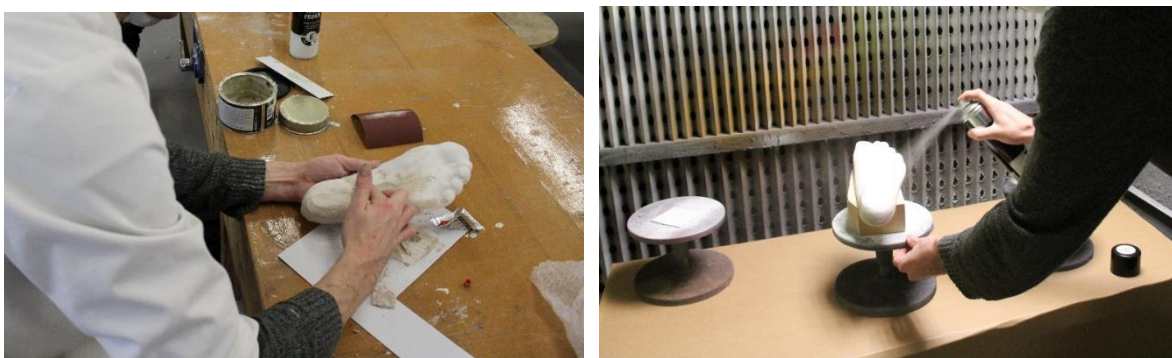
Figure 34: Sanding and priming of plaster cast model (left), Spraying of model (right).
