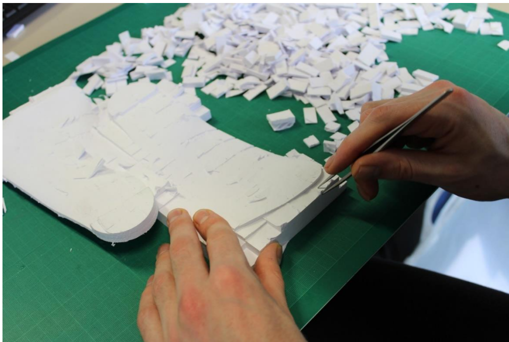
Figure 47: De-cubbing process; removing the part from the solid block of paper.
