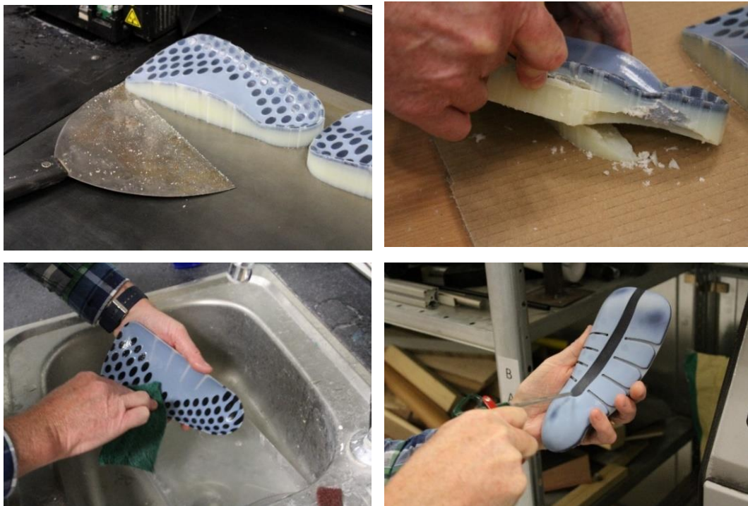
Figure 59: Post processing phase of MMAM orthotic prototypes
