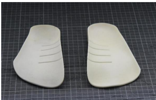
Figure 49: Prototype 2; intrinsic prototypes created using 3DP process
