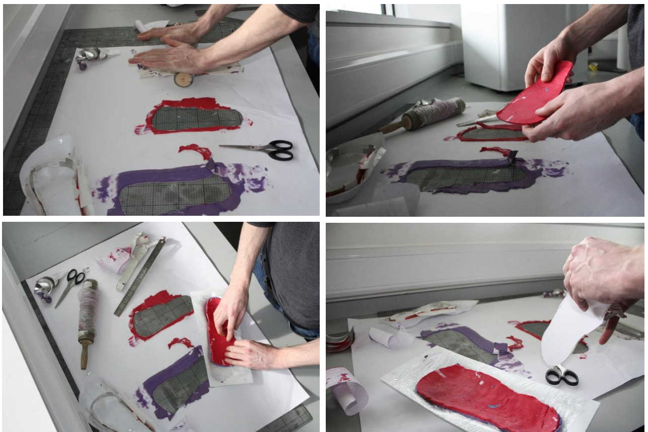
Figure 44: Sketch modelling process, involved using plasticine clay and a negative to create a sketch model, tailored to the foot anatomical features.
