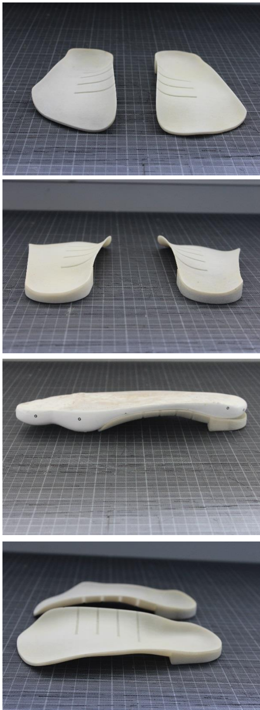
Figure 51: Prototype 1; extrinsic prototypes, fabricated using 3DP powder process.
