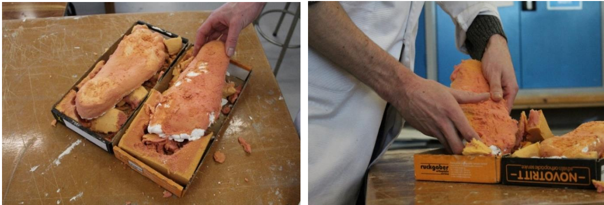
Figure 32: deconstruction of the mould (left), removal of excess orange foam from casting (right)
