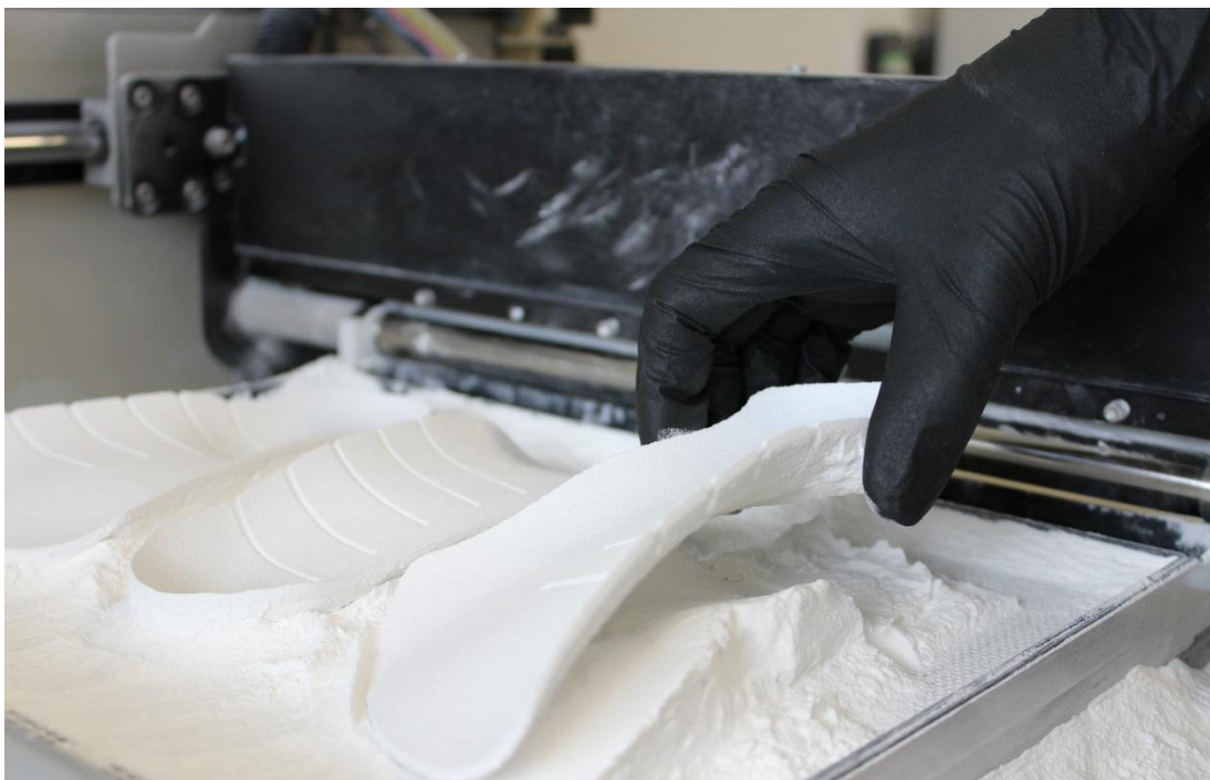
Figure 50: The 3DP post processing phase, of both extrinsic and intrinsic prototypes.
