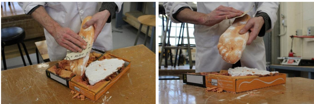
Figure 33: Sanding of the plaster cast model.
