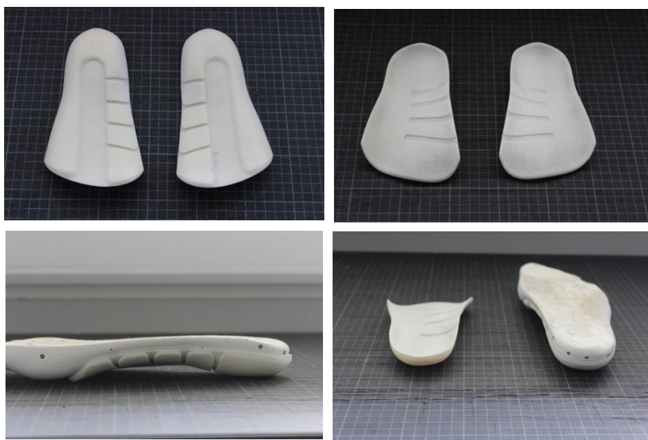
Figure 52: Prototype four; with flex feature and slime posting, fabricated using SLA technology
