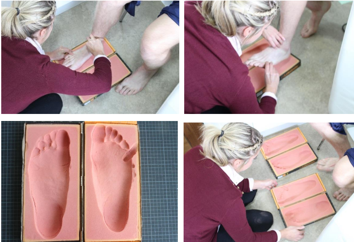
Figure 24: The podiatrist; capturing the optimal positioning of the foot, using the foam impression box.
