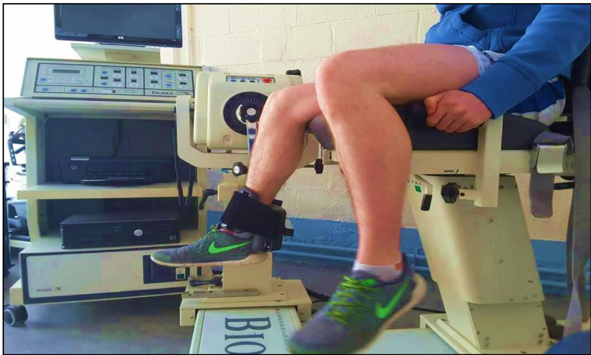
Figure 5: Biodex System 3 eccentric knee flexion apparatus setup.
