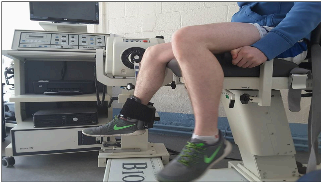
Figure 2: Biodex System 3 eccentric knee flexion apparatus setup.
