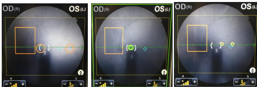
Figure 4.3 - OCT Optimal positioning guide - Orange Circles (Left) = Not Close enough. Yellow Circles (Right) = Too Close. Green Circles aligned (Center) = Optimal position for scan.
