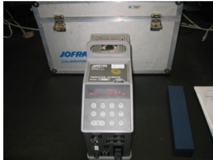
(b) Jofra (D55SE) temperature calibrator
