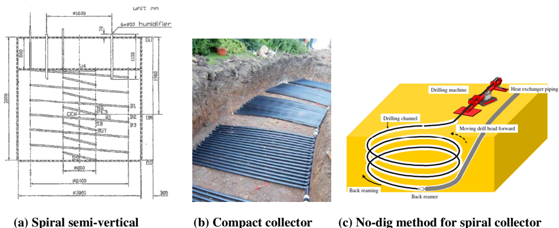
Figure 3-3: New collector designs proposed between 2002 and 2007 (Bi et al. , 2002; Warnelof & Kronstrom, 2005; Hamada et al. 2007)
