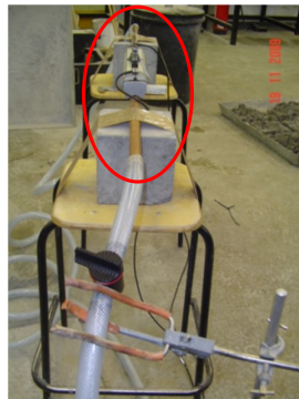
(b) Ultrasonic flow meter probe on copper pipe
