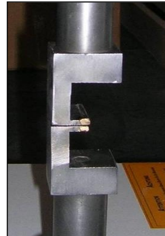
Figure 66: Jig Required for Cleavage Test
