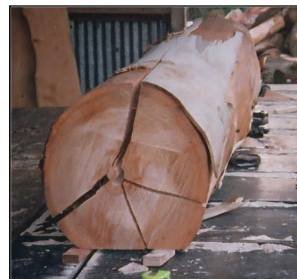
Figure 92: Stem Demonstrating Severe Rupture
