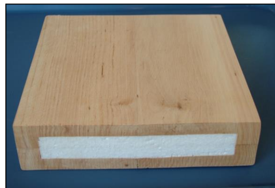
Figure 43: Beehive walls with insulation
