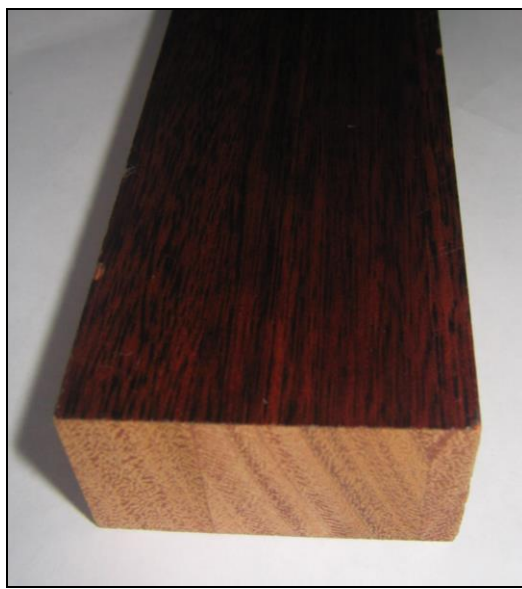
Figure 102: Laminated solid section of eucalyptus with 'tobacco' stain (Courtesy of Lifestyle Furniture)
