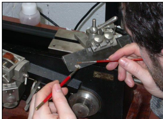
Figure 69: Samples cut on microtome
