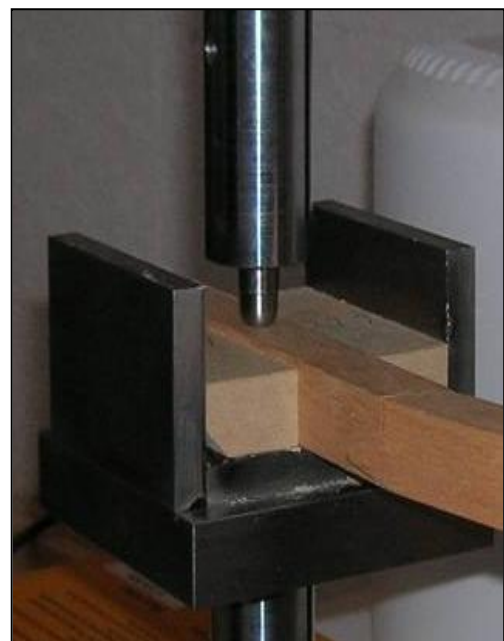
Figure 65: Jig required for Janka Indentation Test
