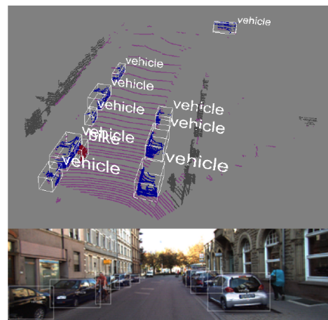
Fig. 3. Sample LIDAR-based bounding box proposals using point clustering. Figure reproduced from [24].
