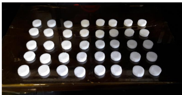
Figure 9. Complete batch of flat-faced tablets produced via FFF 3D printing. Total of 40 tablets covered the print bed of MakerBot Replicator 2X.
