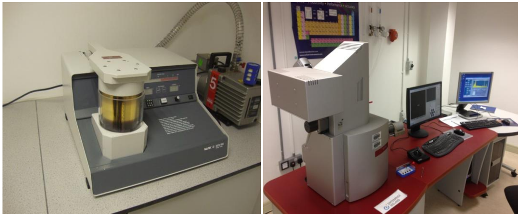
Figure 2.13 Mira scanning electron microscope (left hand side) and Bal-Tec SCD 005 sputter coater (right hand side)
