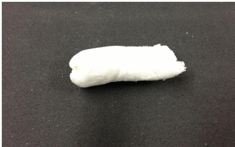
Figure 3.22 Maleic PVA product after freeze drying
