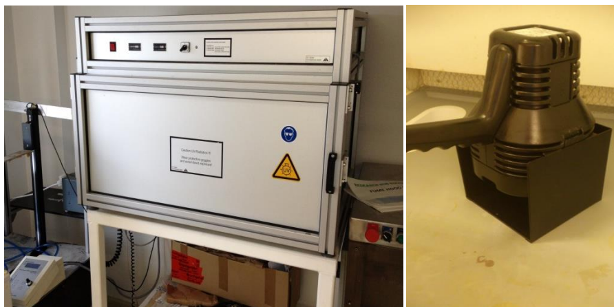
Figure 2.7 Dr. Gröbel UV-Electronik GmbH UV box (left hand side) and UV handheld lamp (right hand side)
