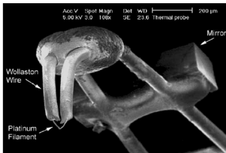
Figure 2.17 Pictomicrograph of a standard probe used for \mu TA.
