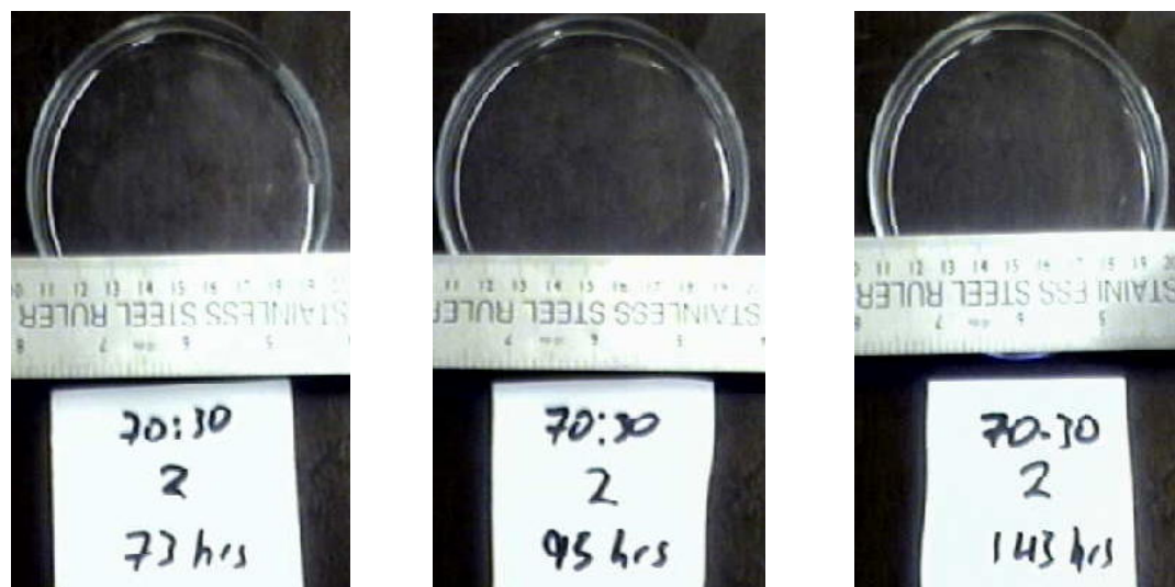
Figure 3.12 Typical swelling characteristics of hydrogel designated 70-30. This sample was swollen in pH7 buffered solution. It should be noted that this sample became transparent after 52hours but did not dissolve until after 143hours.
