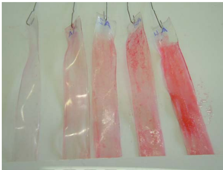
Figure 5.3 Samples coated with 70-30 copolymer crosslinked with 0.1wt% EGDMA. From left to right: no coating; 1 coating cycle; 2 coating cycles; 3 coating cycles; and 4 coating cycles.
