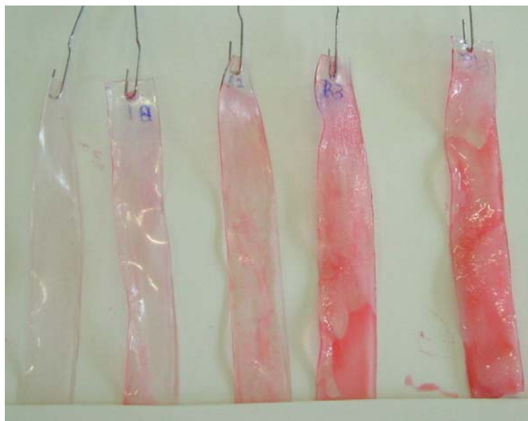
Figure 5.4 Samples coated with 70-30 copolymer crosslinked with 0.1wt% PEG600DMA. From left to right: no coating; 1 coating cycle; 2 coating cycles; 3 coating cycles; and 4 coating cycles.
