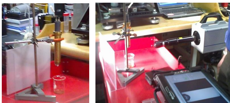
Figure 2 Drophead with the capillary tubing connected at the top (on left). Drophead with the extended camera lens and a screen image(on the right)
