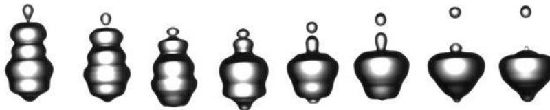
Figure 7 Images of the separation of the satellite drop d2 into d2-1 and d2-2. Frames 405, 406, 407, 410, 412, 413, 416, 417.
