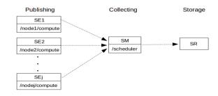
Fig. 2. Service Discovery Procedure
