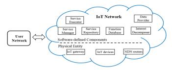
Fig. 1. System Components
