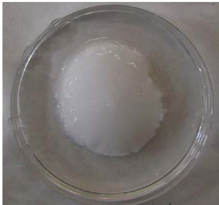
Figure 1 A picture of a PVA/NaOH/H 2 O gel formed by the process described in the text
