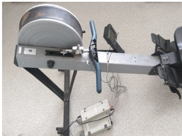
Figure 1 – Rowing ergometer custom fitted with a load cell for the 7SM test.
