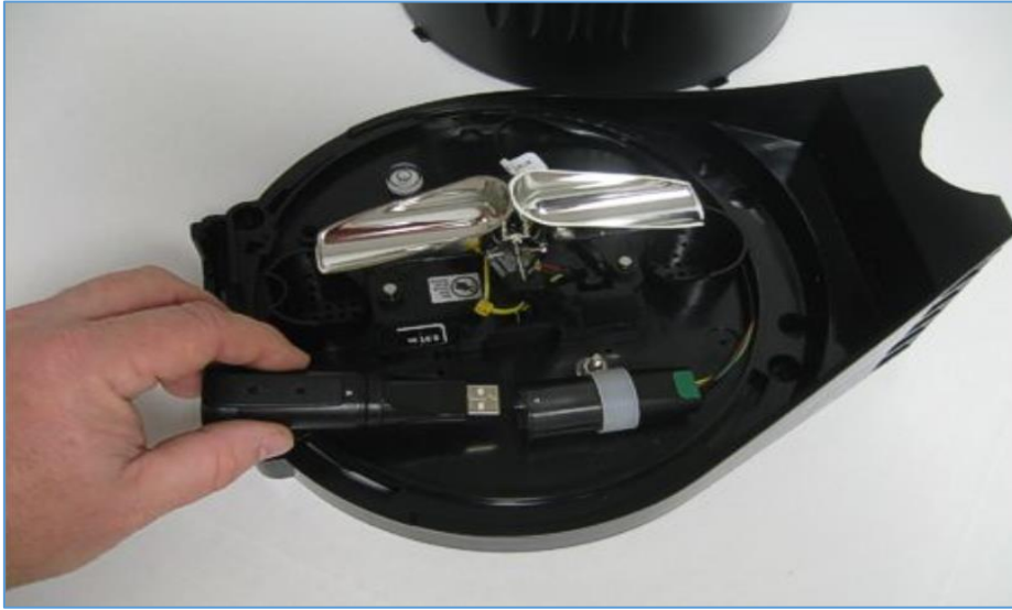
Figure 51: Inserting data-logger into the base of the rain gauge. Source: www.weathershop.com
