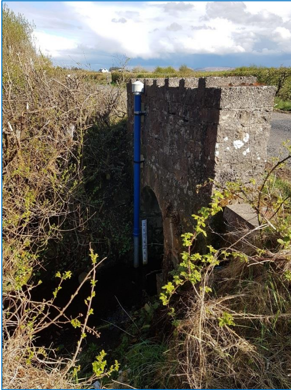
Figure 43: MP7 with its water-level data-logger in-situ.
