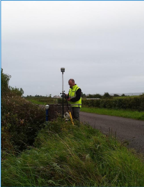
Figure 48: Using a Trimble® receiver & network to survey & establish a temporary bench mark (TBM) at MP7.
