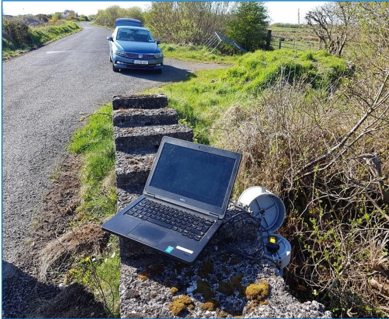
Figure 46: Set-up & interrogation of the data-logger/ITC using OTT software
