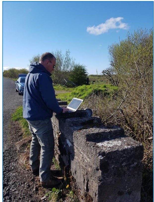
Figure 47: Set-up & interrogation of the data-logger/ITC using OTT software
