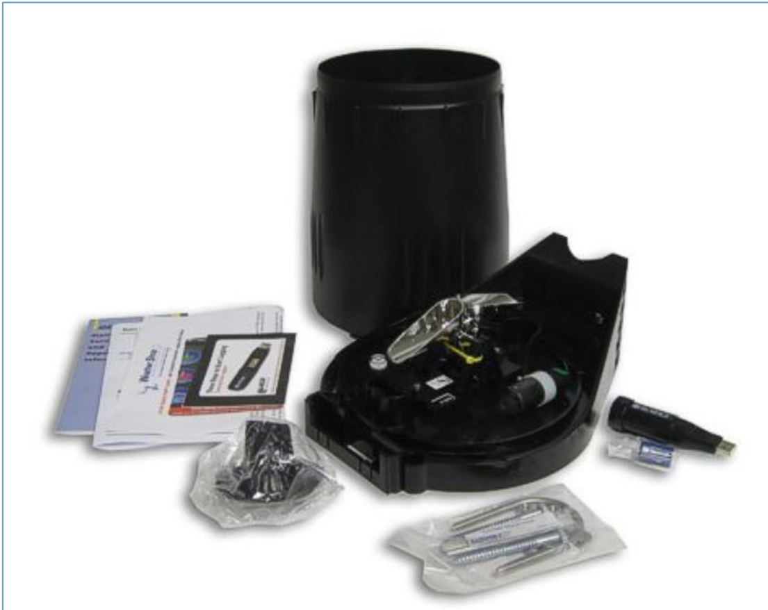
Figure 50: Davis Instruments® self-contained automatic logging rain gauge with rain cone in background and base with bubble level and tipping spoons in foreground. Source: www.weathershop.com
