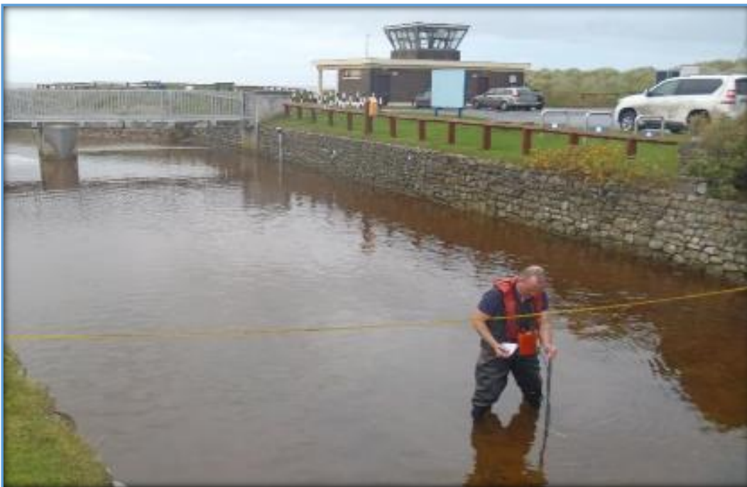
Figure 38: Velocity measurement by current meter at one of the vertical points along a cross-sectional area of the river
