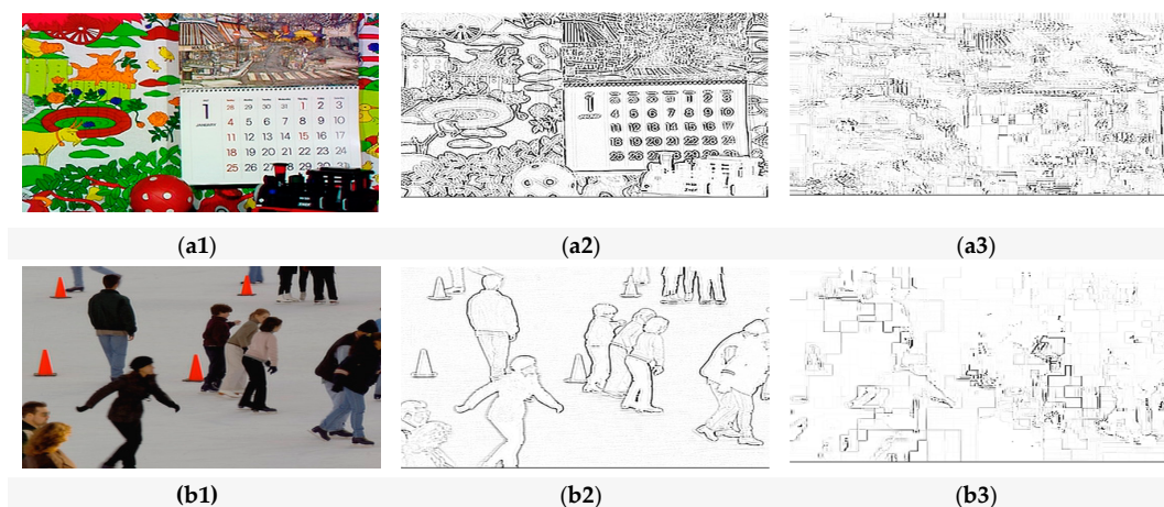
Figure 6. The comparative visual impact of EXPer on ICE and mobile video sequences after Laplacian edge detector. (a1) Plaintext mobile video frame; (a2) detected edges of plaintext mobile video frame; (a3) detected edges of encrypted mobile video frame; (b1) plaintext ICE video frame; (b2) detected edges of plaintext ICE video frame; (b3) detected edges of encrypted ICE video frame.
