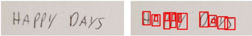
Figure 3.11: On the left, an image of a handwritten label. On the right, the detected contours with red rectangles drawn around them. The image on the right highlights the first challenge of extracting the characters from a handwritten label. Multiple parts of a single letter are being detected. This can be seen where a rectangle is contained within another rectangle.
