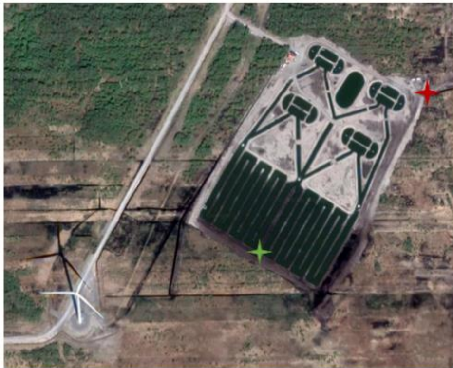
685 686 Figure 1: A) Schematic of trial fish farm, located in Ballycon, Co. Offaly. 1, 2, 3 & 4) Split Ponds for culturing, 5) 687 Water Reservoir, 6) Algae & Duckweed Treatment Channels, 7) Holding Tank, 8) Bog River (intake source). 688 Black lines indicate the direction of the flow of water. Black boxes indicate the locations of the paddle wheels. 689 NOTE: Schematic is not to scale. B) Aerial view of the trial fish farm within the peatlands. The wind turbine used 690 to provide all electrical needs for the farm is included. The D-ends of each split pond can be seen. The red stars 691 indicate the location of the intake sampling point. The green stars indicate the location of the holding tank 692 sampling point.
