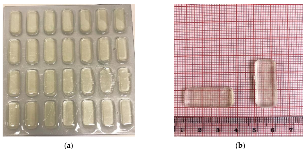
Figure 3. (a) Complete batch of printed dosage forms fabricated via SLA 3D printing ( n = 28 ) (b) single dosage form.
