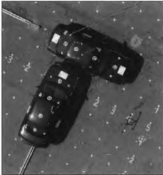
Photograph 4.3 The arrangement of targets placed on the vehicles and the indexing system in the surrounding area (Coyle, 2003).
