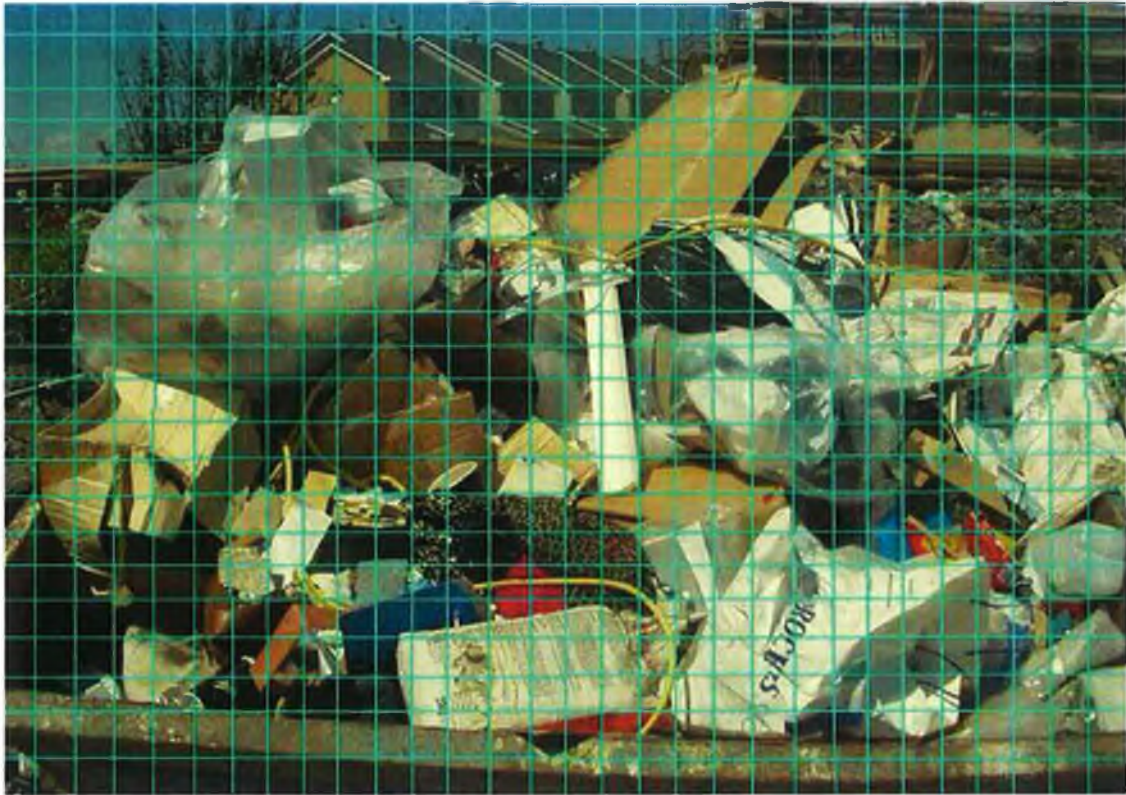
Photograph 5.3 The effect of a superimposed grid and its density on the photographic analysis
