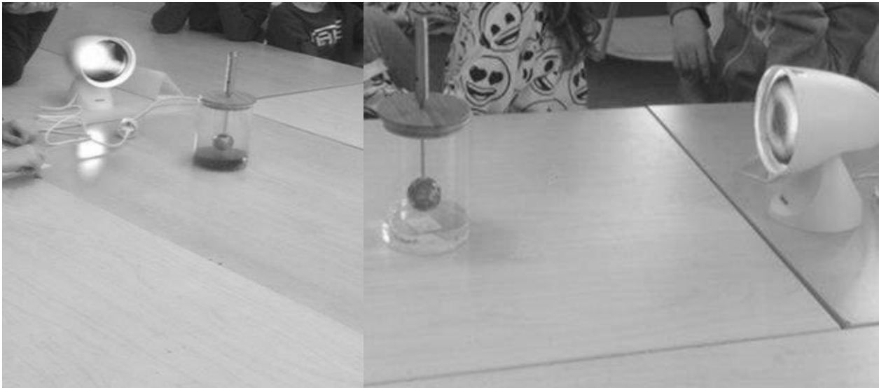
Figure 1 and 2. One lamp (the sun), one glass jar with lid (greenhouse), a thermometer fixed in a small globe (the earth). To the left, pink fluid (c-vitamin (CO 2 )) and water, to the right only water. Two comparative experiments that were continuing at the same time.
