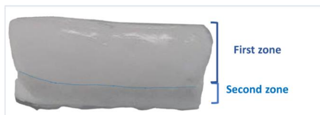
Figure 4. Macroscopic evaluation of the cryogel after production. The dashed line represents the two different regions perceived.
