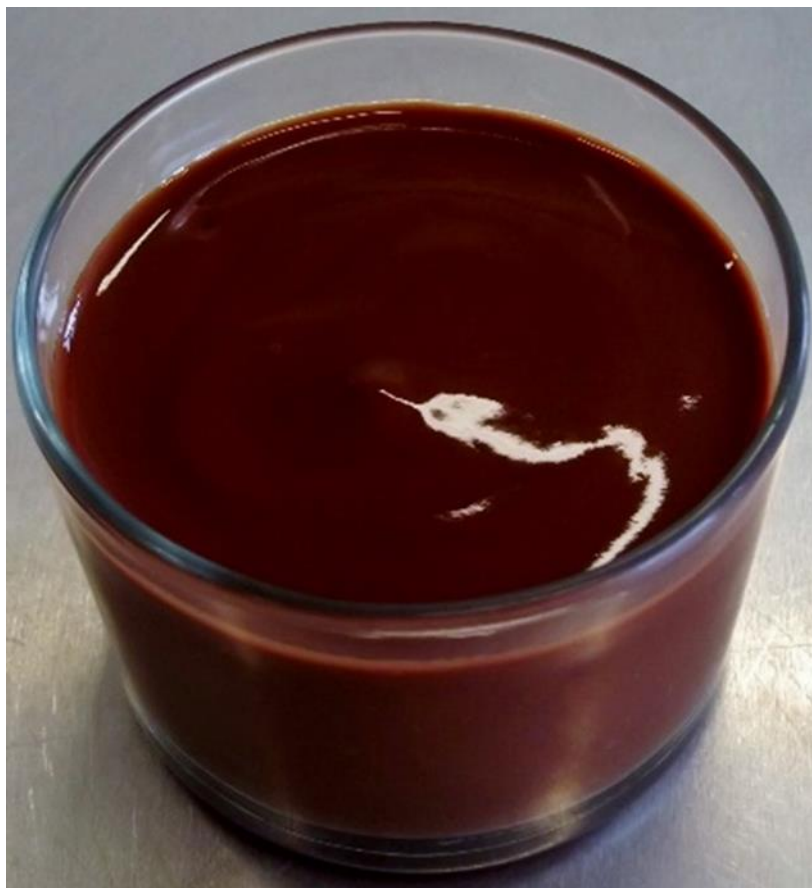
Figure S.2. Nanosuspension of pinhão seed coats after 30 steps through the mechanical mill.
