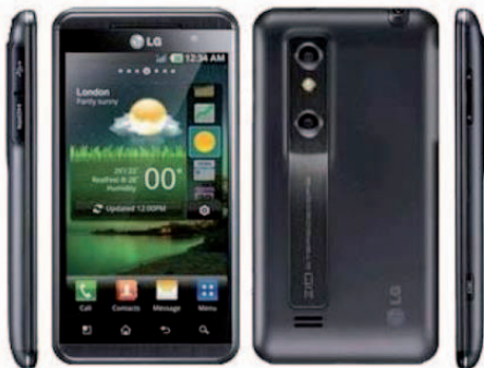
Fig. 3. LG Optimus 3D mobile phone equipped with parallax-barrier based autostereoscopic 3Dscreen and stereo camera
