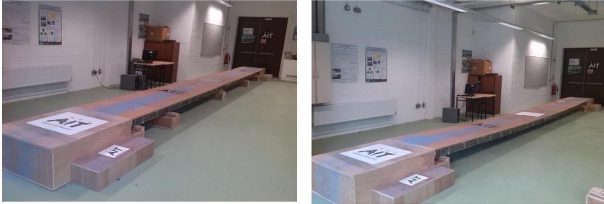
Figure 8. Left, footbridge set-up for rigid walking; right, flexible footbridge set-up
