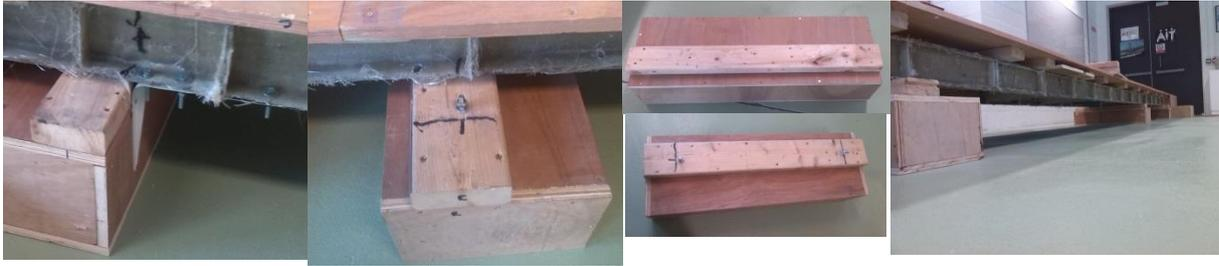
Figure 5. Left, pin connection for 8m span; centre left, opening and arrangement for pin connection for 6.5m to 7.5m spans; centre right, roller support top, and pin support bottom; right, rigid support arrangement
