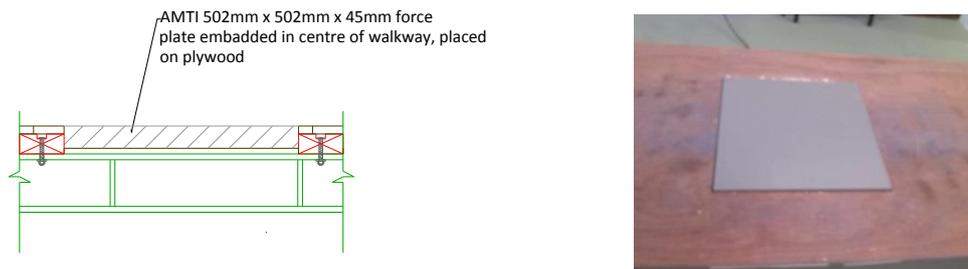
Figure 6: Left, schematic detail of embedded force plate (not to scale); right, actual force plate
