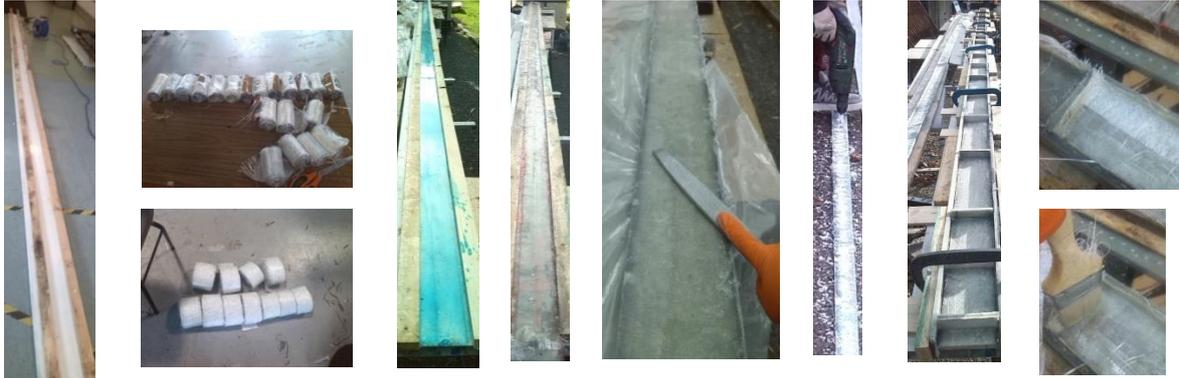
Figure 2. Left 9m long mould; 2<sup>nd</sup> left, 9m lengths of WR and SM prepared; 3<sup>rd</sup> left, mould coated with PVA release agent; left centre, finished plank; right centre, plank's rough edges being filled off; 3<sup>rd</sup> right, 5mm borings in flanges; 2<sup>nd</sup> right I-Beam with cleats glued and held to set using G-clamps; right, I-beams reinforced with woven rovings and shredded mat
