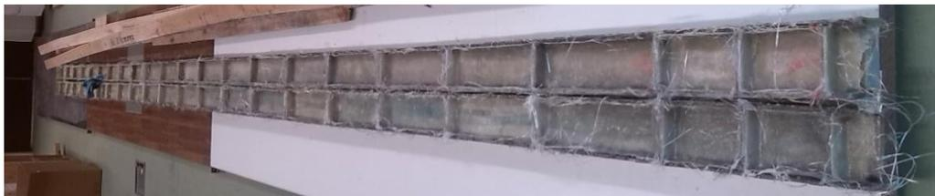
Figure 3. Finished 9m long I-beams
