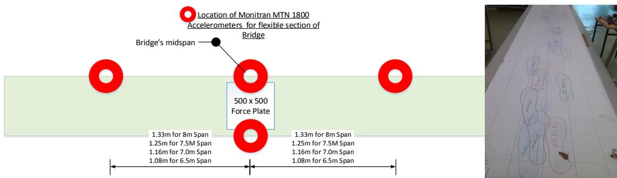
Figure 7: Left, location of accelerometers on bridge; right, grid paper ready to be measured
