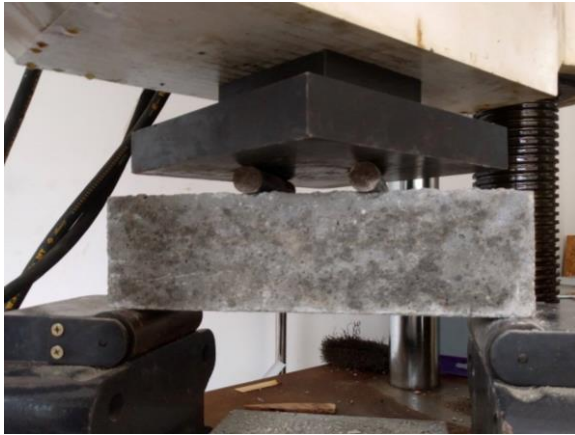
Fig. 2 : Testing Beam specimens for flexural strength.
