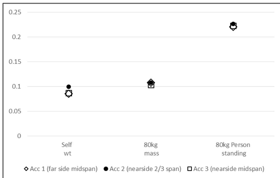
Figure 5. Logarithmic Decrement for Empty Structure and Test Scenarios involving inert mass and humans at midspan.
