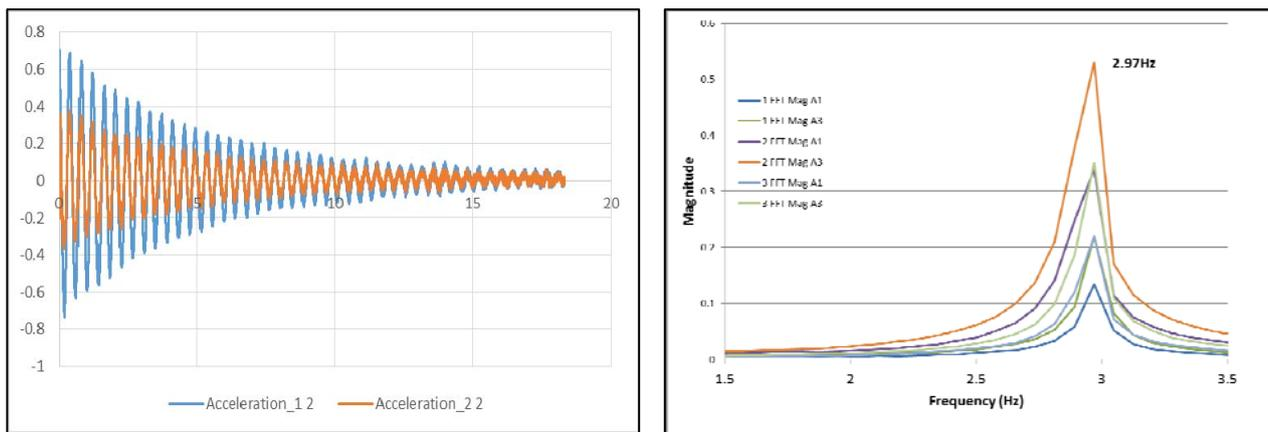
Figure 3. (a) Acceleration response of 8.0m span under self-weight (b) FFT of acceleration traces for 8.0m span under self-weight
