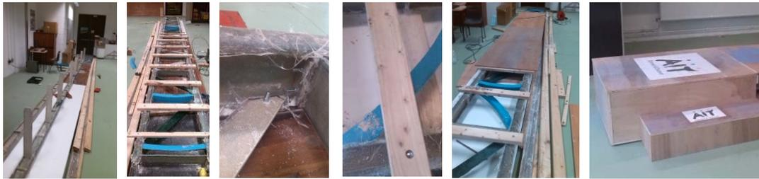
Figure 1. Construction of the Laboratory Scale FRP Composite Footbridge
