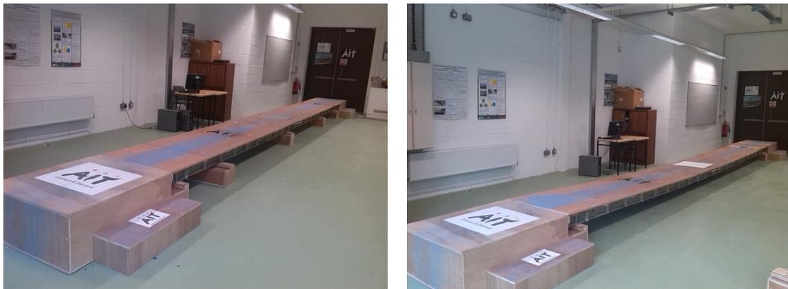
Figure 2. Completed Laboratory Scale FRP Composite Footbridge
