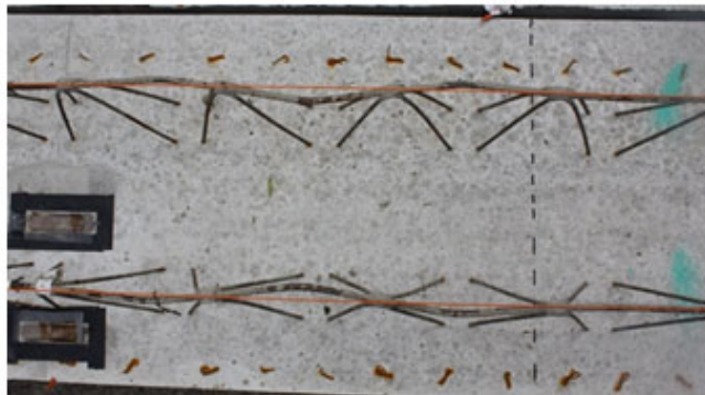
(c) buckling of top chord between diagonals (W22.5-08/05/05)
