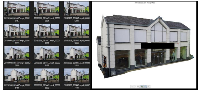
Figure 2-Photogrammetry as a technique to create realistic 3D content based on photos.
