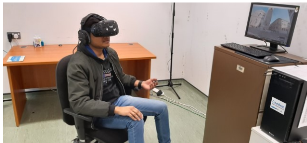
Fig. 1. Test subject wearing Vive HMD with integrated Tobii eye-tracker watching source stimuli. E4 wristband is strapped on wrist to record EDA
