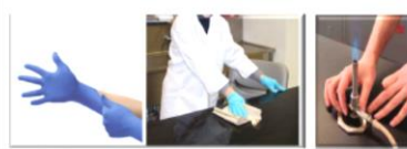
Wearing PPE, ensure work space is clear and clean. Carefully light bunsen.
