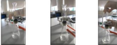
Turn on suction and allow sample to completely filter through. Gently remove column.
