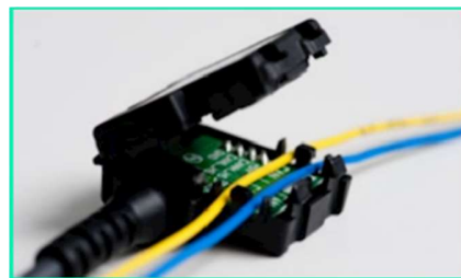
Figure 3: Contactless CAN clip. CAN-High and LOW wires pass through the clip, in which all CAN signals are sensed and transmitted to FMS Gateway
