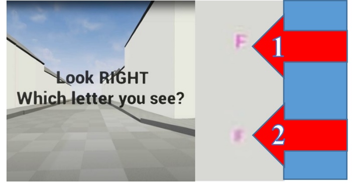
Fig. 3- Training section and zoomed letters representing the minimum resolution requirements (1) and outside limits (2).
