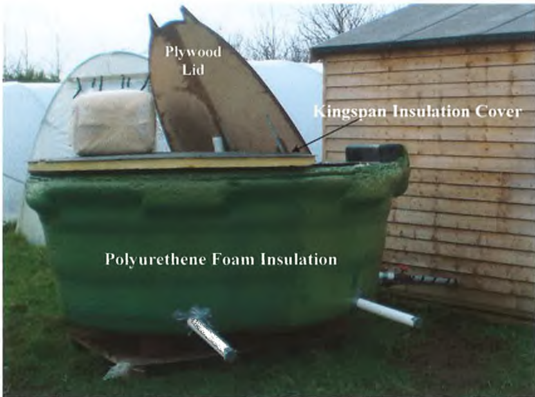
Figure 2.13: HEU showing the external polyurethane insulation and the 50mm Kingspan insulation lid with perspex cover.
