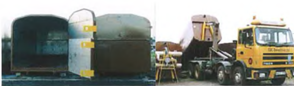
Figure 2.6: Aergestor system roll on roll off.
