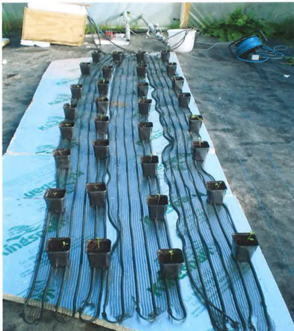
Figure 3.6: 'Roll n Grow' heating mat setup within the polytunnel with Kingspan insulation underneath and 8 replicates of each plant.
