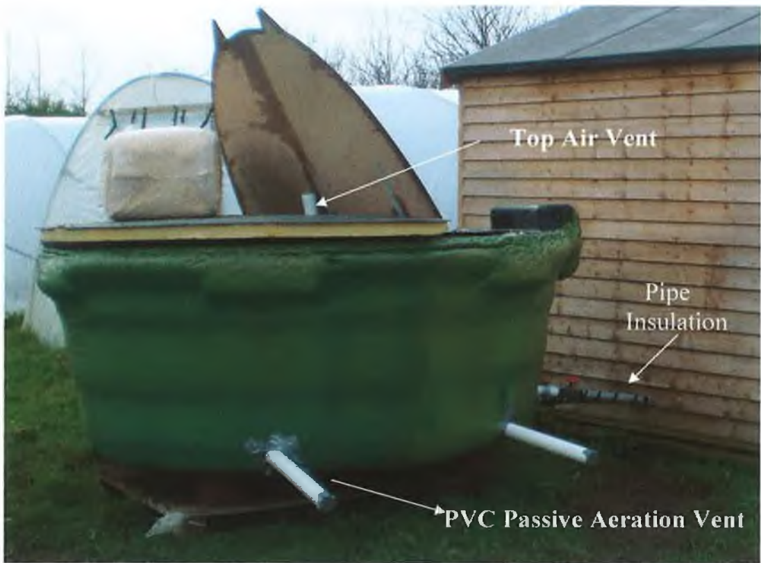
Figure 2.33: External view of full scale experimental design with passive aeration pipe work and top air vent highlighted.
