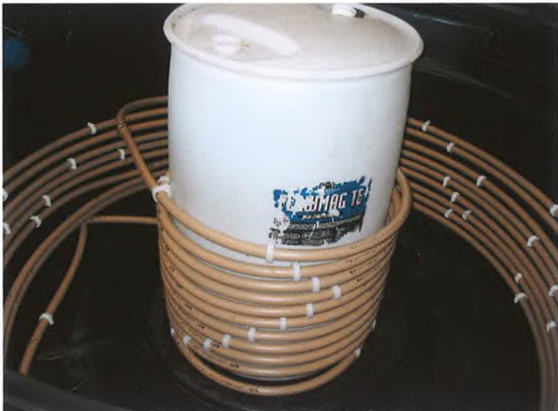
Figure 2.11: Qualpex piping setup inside the HEU for heat extraction experiment.
