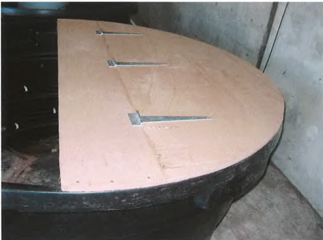
Figure 2.10: Example of the removable Marine Plywood Lid constructed to cover the 2046 litre trough (HEU).
