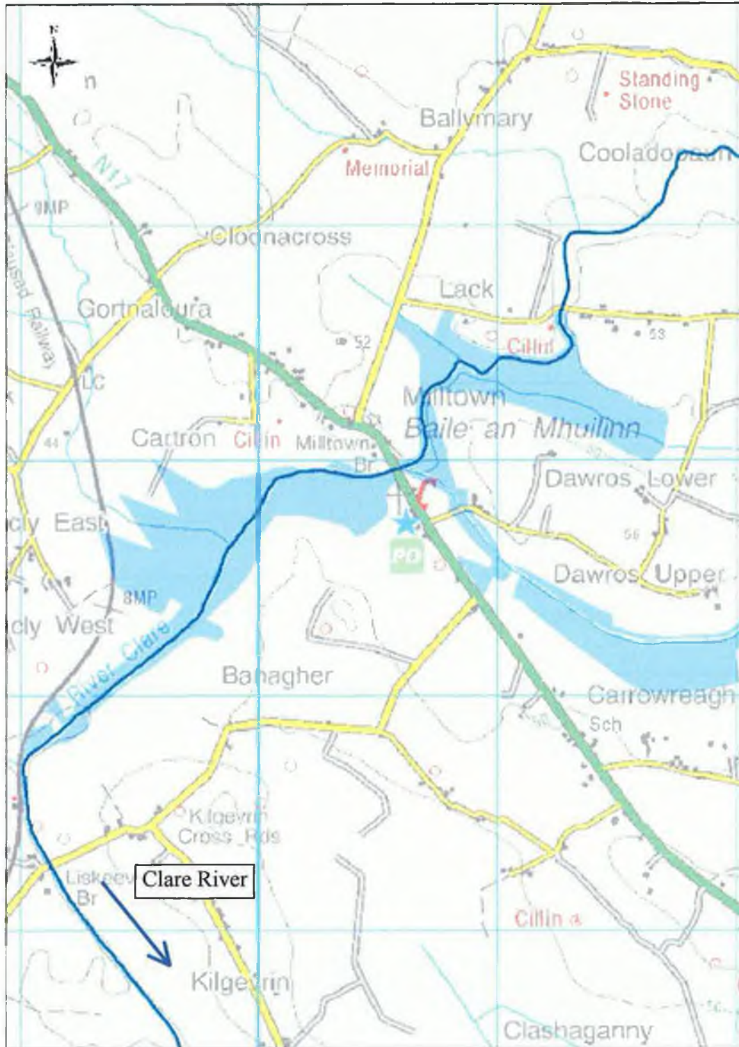
A-2.6 – Flood Extent Map for Clare River at Milltown for November 2009 Flood Event
