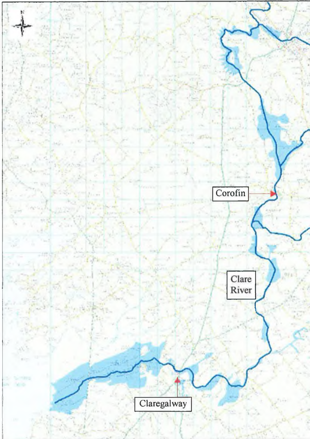
A-2.1 – Flood Extent Map for Clare River from Tuam to Lough Corrib for November 2009 Flood Event
