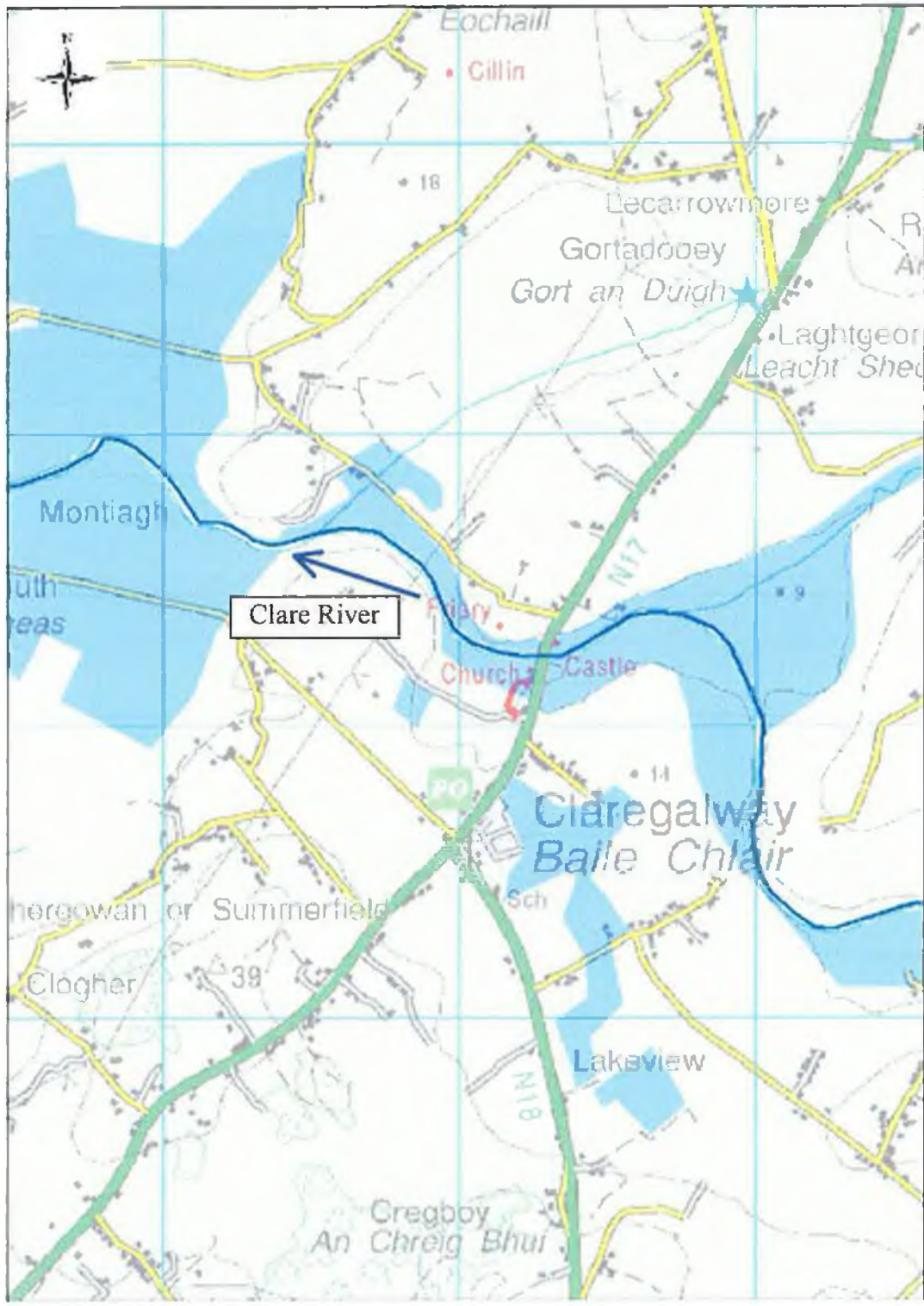
A-2.2 – Flood Extent Map for Clare River at Claregalway for November 2009 Flood Event
